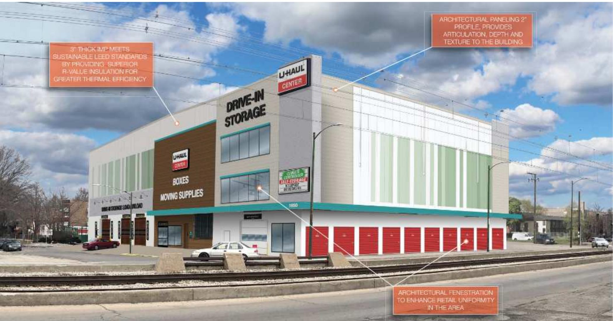
3" THICK IMP MEETS SUSTAINABLE LEED STANDARDS BY PROVIDING SUPERIOR R-VALUE INSULATION FOR GREATER THERMAL EFFICIENCY
